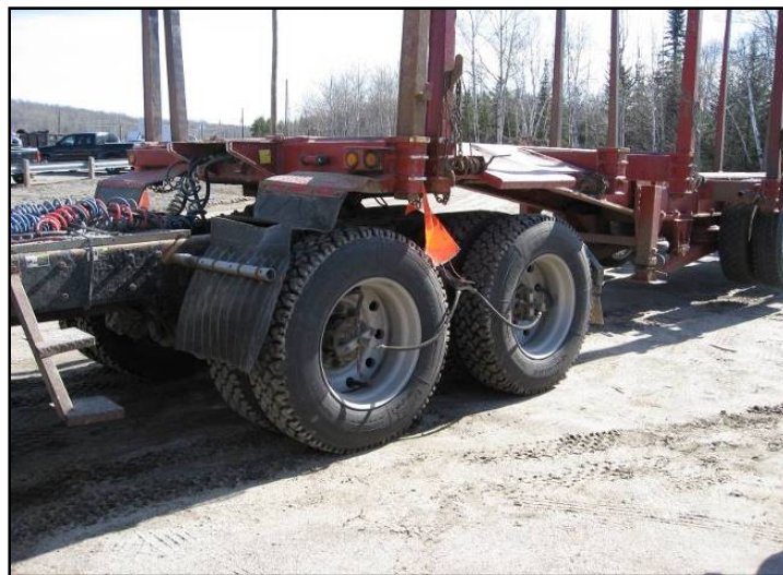
Figure 5.3: A typical TPCS equipped logging truck on Highway 651
