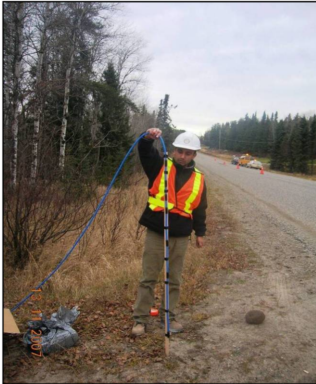
Figure 4.1: View of Thermistor String at Test Site
