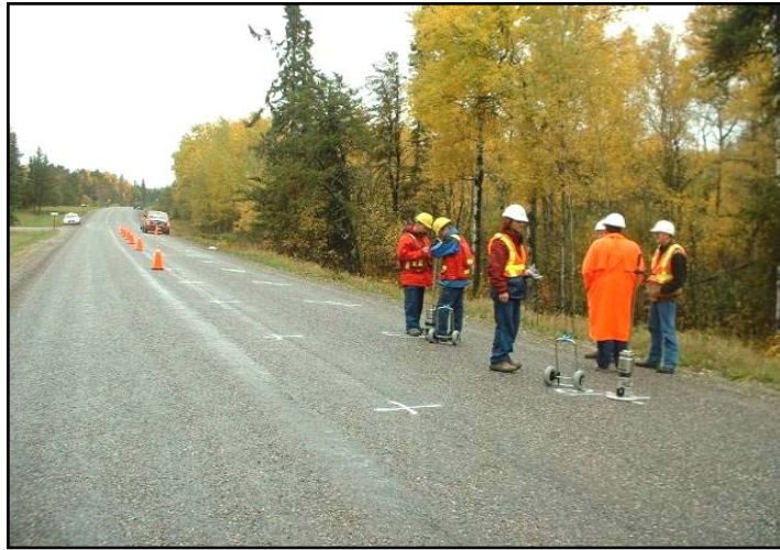
Figure 3.9: Test Section on Hwy 601, PFWD Testing in Progress
