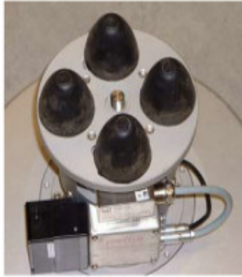
Figure 3 : rubber buffers and load cell
