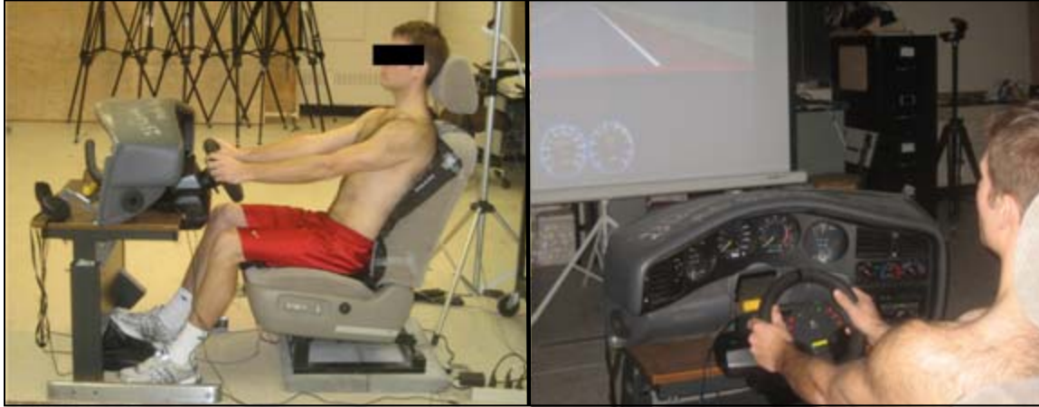
Figure 2: Driving simulator set up. Seat with pressure mapping system, pedals and steering wheel (Left), occupant's view of simulated road (Right).
