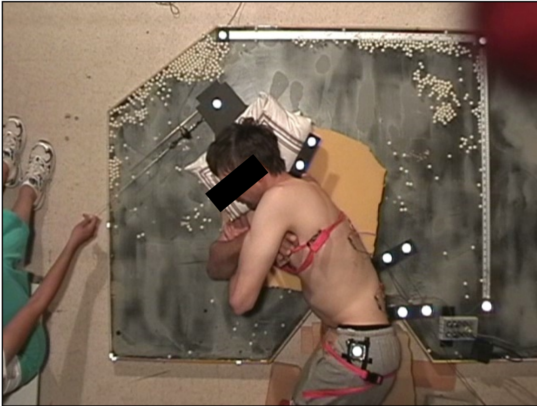
Figure 6: View of passive lumbar flexion measurement from video camera fixed to the ceiling directly over the participants. LED trigger light, used to synch coordinate data with EMG and force data, can be seen in the upper right hand corner of the image.
