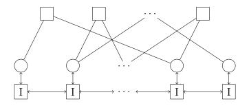
Figure 4.6: Message passing diagram of LDPC Decoding over finite-state channels
