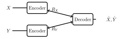
Figure 2.1: IED scheme for the separated encoders and the joint decoder
