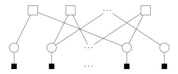
Figure 4.3: General LDPC Decoding for memoryless channels
