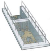
1. Upon entering the plant, wastewater is pumped through bars or screens to remove large debris such as newspapers, sticks, rags, and cans.
