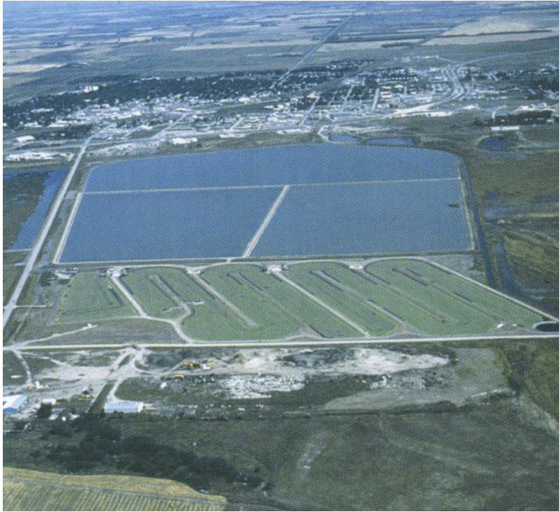
4.14 | Devil's Leg Waste Water Treatment Plant A 20 hectare waste treatment plant situated at Devil's Lake, North Dakota, USA, in a former wetland environment. Now, this system treats waste water using biological processes associated with a proprietary system utilizing floating aquatic plants that survive in all climates. Duckweed plants absorb and neutralize pollutants in the water, as well as stabilize biological processes in the pond, as was designed and intended by Viet Ngo/Lemna International.
