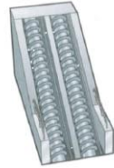
2. Sewage pumps lift the wastewater to primary settling tanks at surface level.
