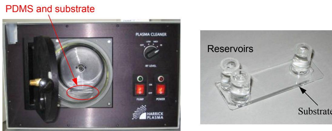
Figure 3.2: Plasma treatment system and a typical bonded chip.
