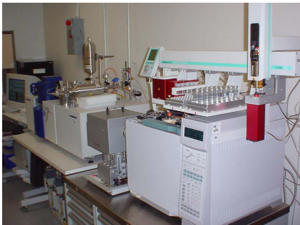
Figure 2.2 The CF-IRMS system attached to the gas chromatograph which is equipped with an autosampler.
