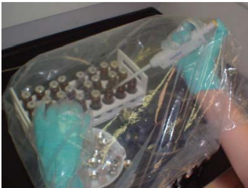
Figure 2.4 Methyl iodide is added to samples in an inflatable glove bag connected with an ultra pure helium tank.
