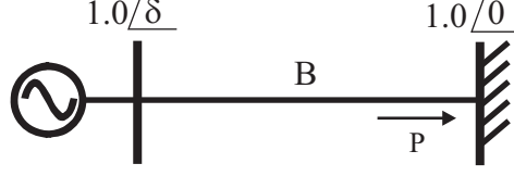
Figure 3.3: Generator-Infinite Bus system
