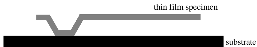
Figure 3-3- Micro fabricated thin film specimen anchored on the substrated.
