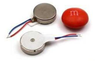
Figure 14: VMP2 tactor. Image source: Solarbotics (2007).
