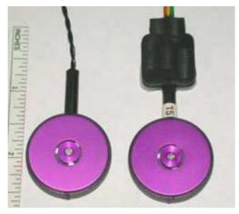
Figure 12: C2 Tactor. Image source: Engineering Acoustics, Inc. (2007).
