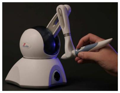
Figure 2: PHANTOM Omni. Image source: SensAble Technologies (2007).
