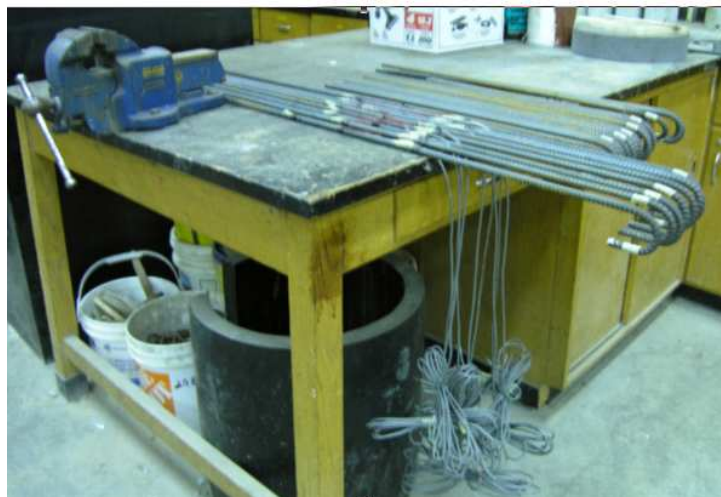
Figure 3.24 Strain gauges attached on rebars
