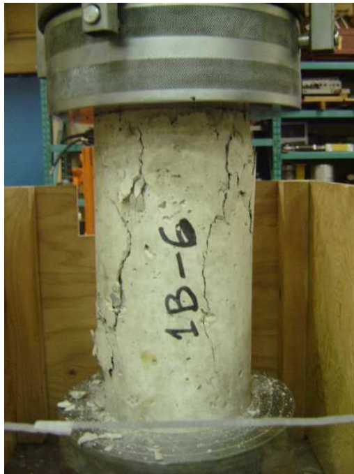
Figure 3.12 Crushing of the concrete cylinder #6 (6"x12") of the first batch concrete
