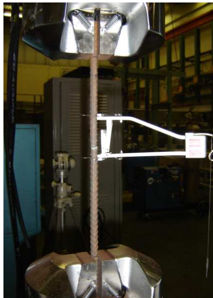
Figure 3.16 Testing of original rebar
