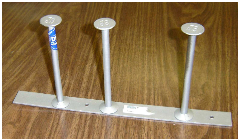
Figure 2.3 Headed shear studs welded to a bottom steel plate
