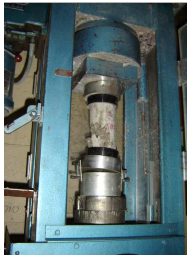
Figure 3.9 Compression test of the concrete cylinder (4”x8”)
