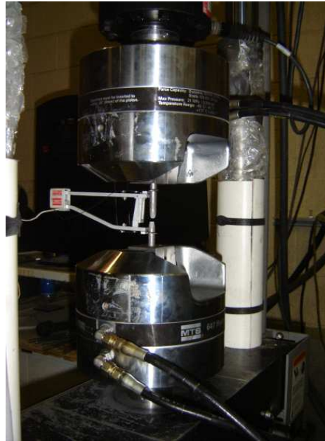
Figure 3.20 Testing of the original bolt
