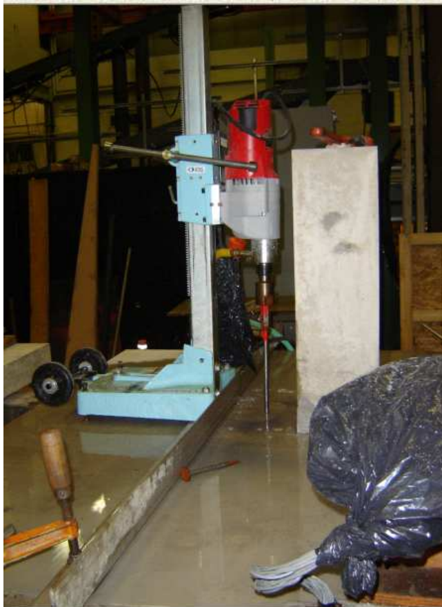
Figure 3.31 Drilling holes in the slab
