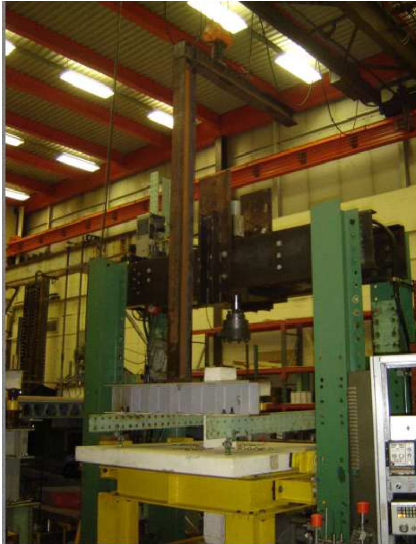
Figure 3.43 Lifting of the concrete specimen
