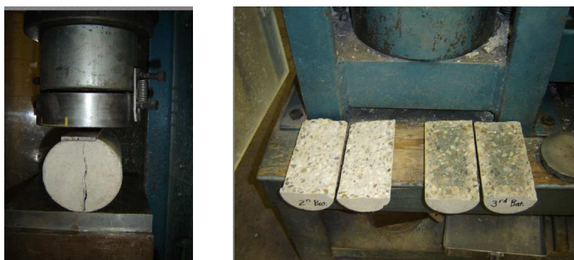
Figure 3.10 Concrete cylinder tension test
