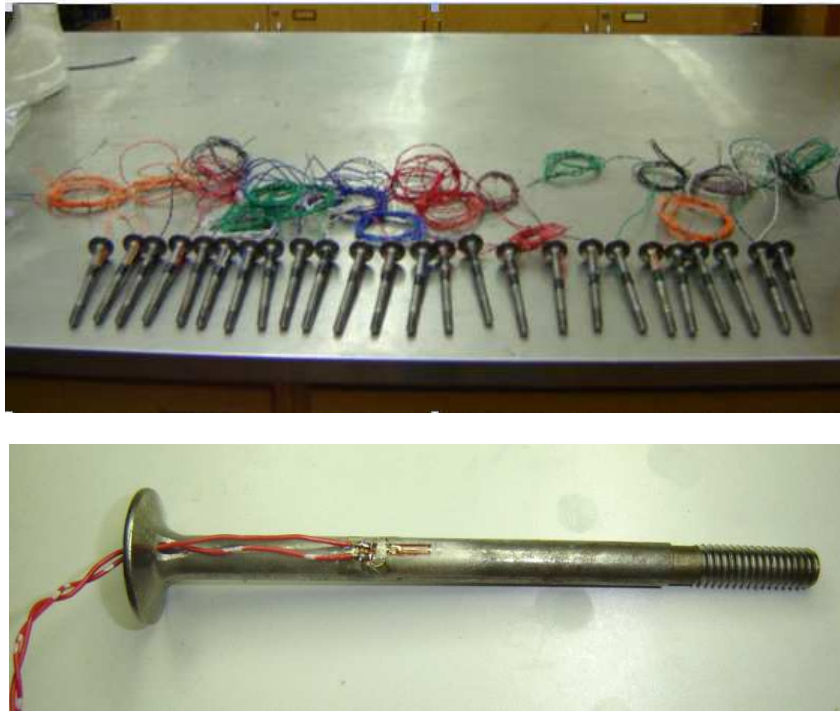
Figure 3.30 Shear bolts with strain gauges
