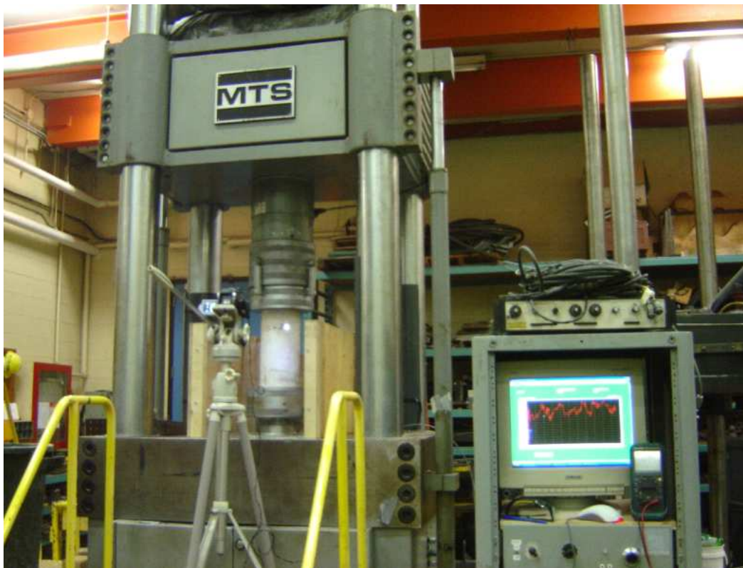
Figure 3.11 Concrete cylinder (6"x12") compression test
