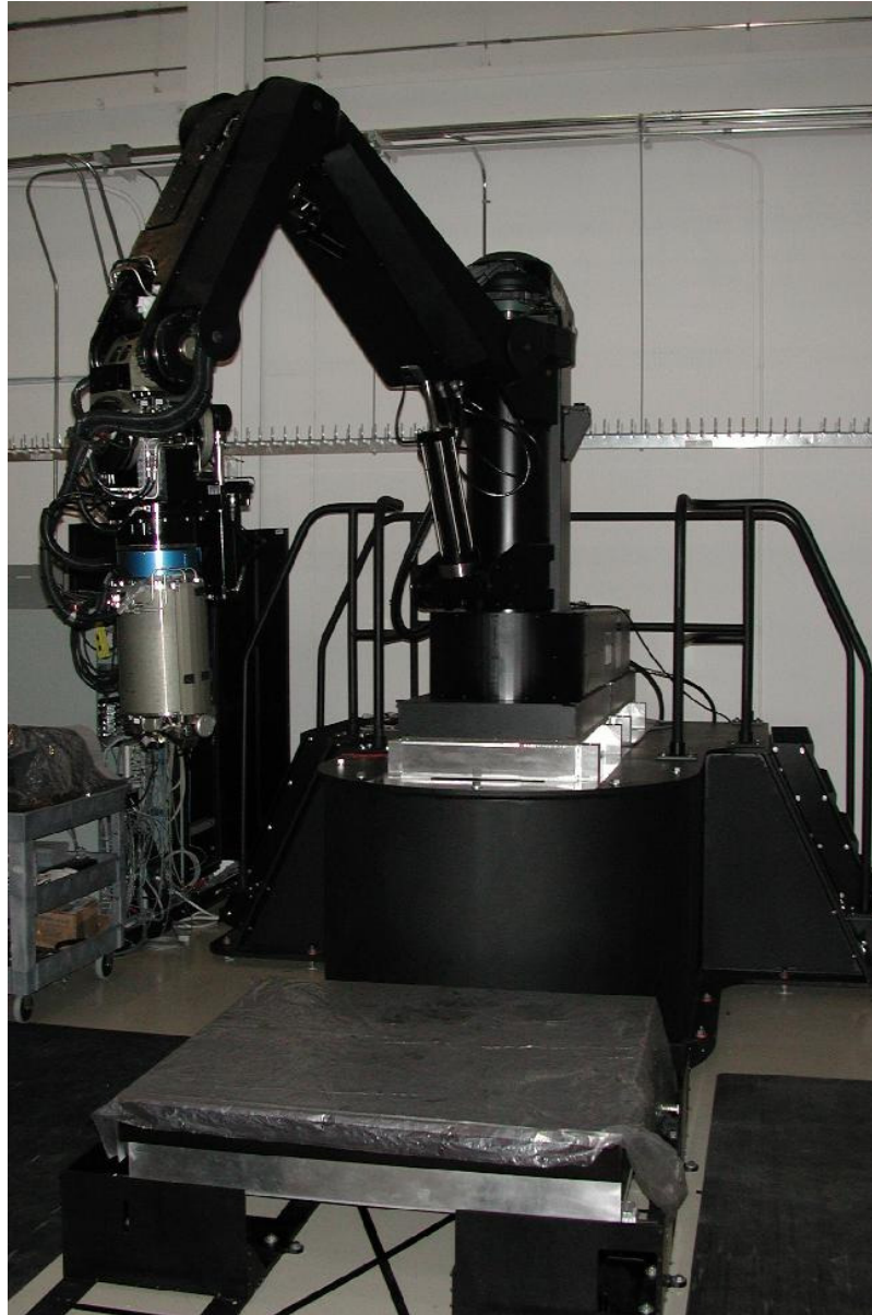
Figure 5.23: The SMT and the worksite force-plate.
