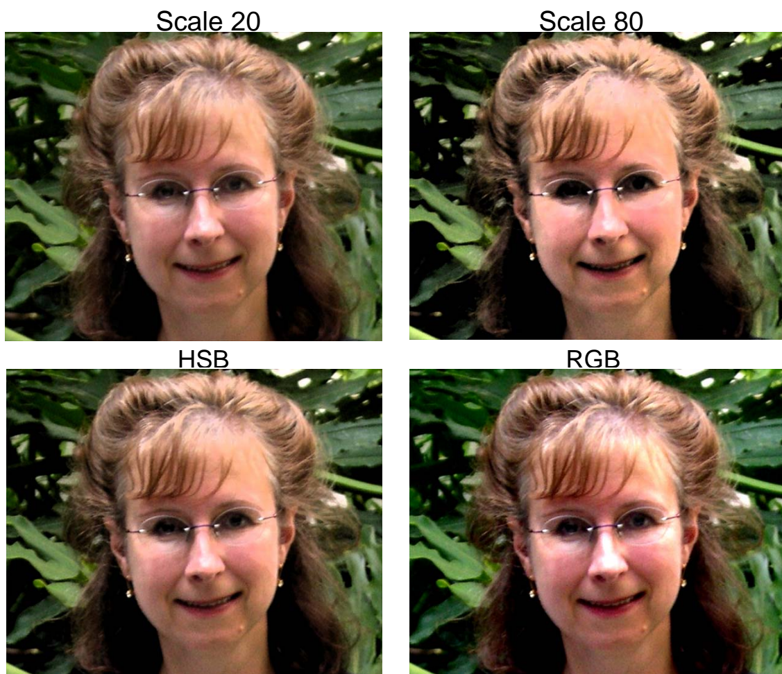
Figure 6-12. Face images enhanced with the contrast enhancement filter in two scales (20 and 80) and two modes (HSB and RGB).
