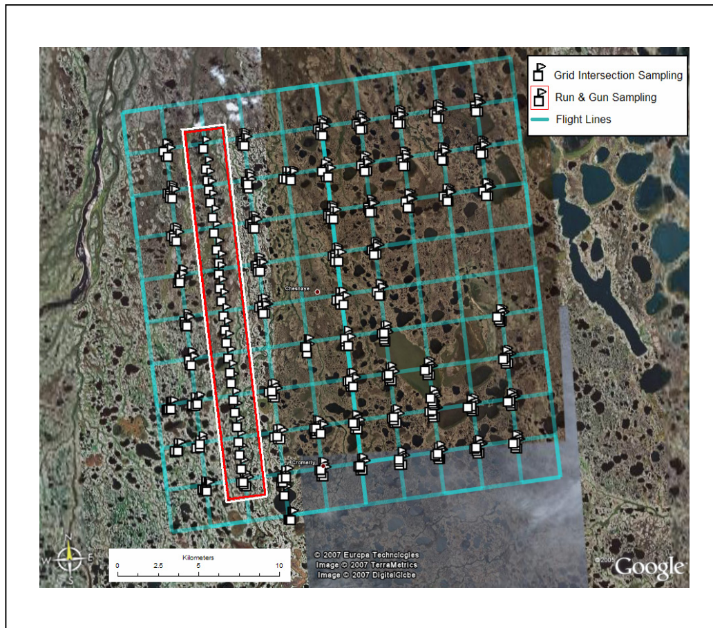
Figure 4.2 Tundra study site flight grid and snow survey locations with a Google Earth™ background image.
