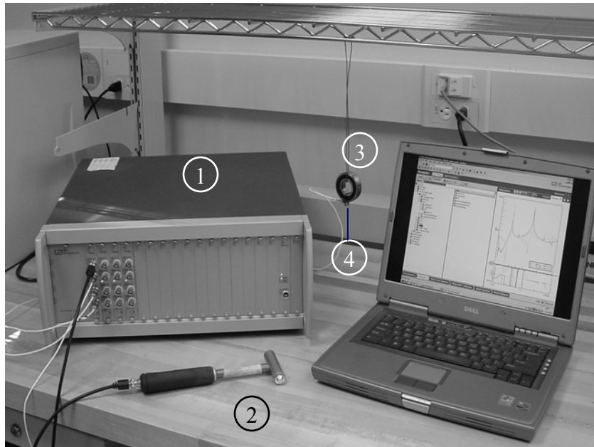
1. SCADAS III 2. Impact hammer 3. Test bearing 4. Accelerometer
