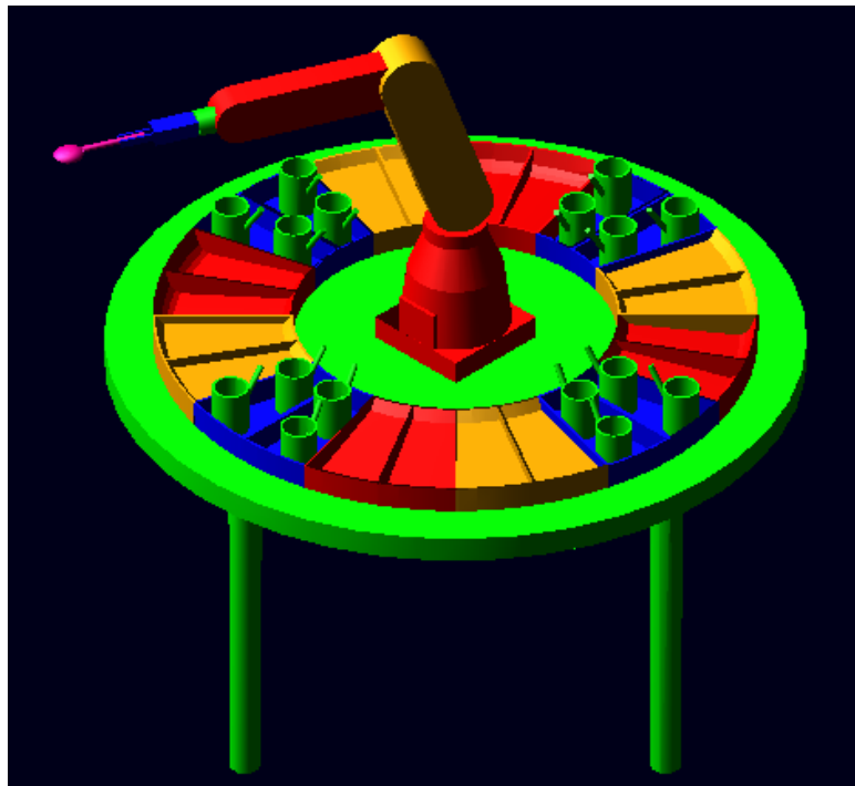
Figure 4-8: 3D model of the robot located in the center of the table along with four food trays.
