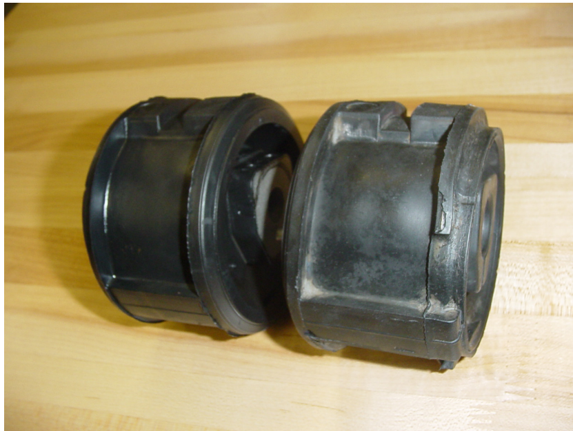
Figure 9-2: A healthy hydraulic bushing (left) and a defected bushing with the MR fluid (right)
