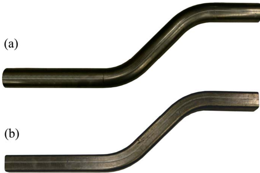
Figure 24: Comparison of (a) a non-hydroformed s-rail and (b) a hydroformed s-rail
