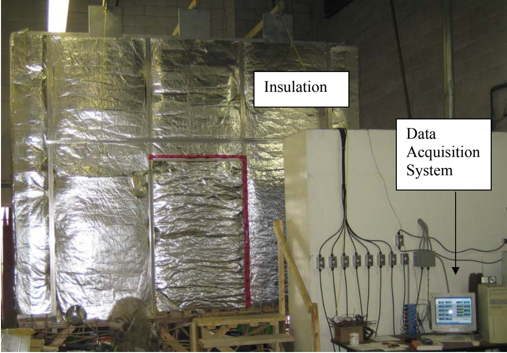
Figure 3.9: Overall View of Completed Radiant Panel Test Facility
