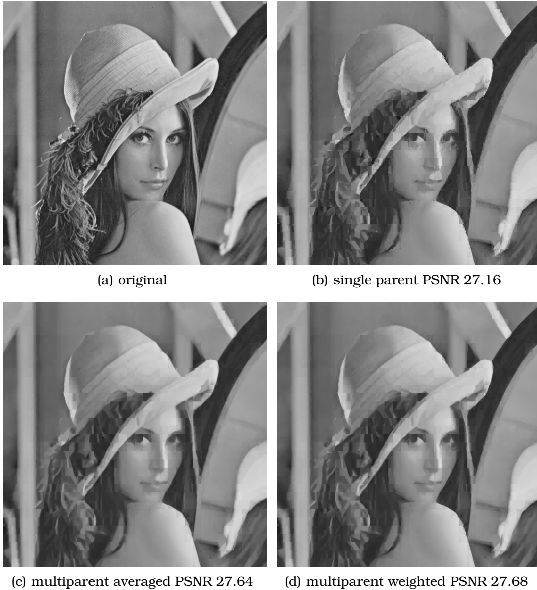
Figure 3.20: Lena partitioned into 16 \times 16 pixel range blocks. a) original b) estimated by a conventional IFS scheme c) averaged result over 10 parent blocks d) weighted average ( as 1/err^4 ) of 10 parents.
