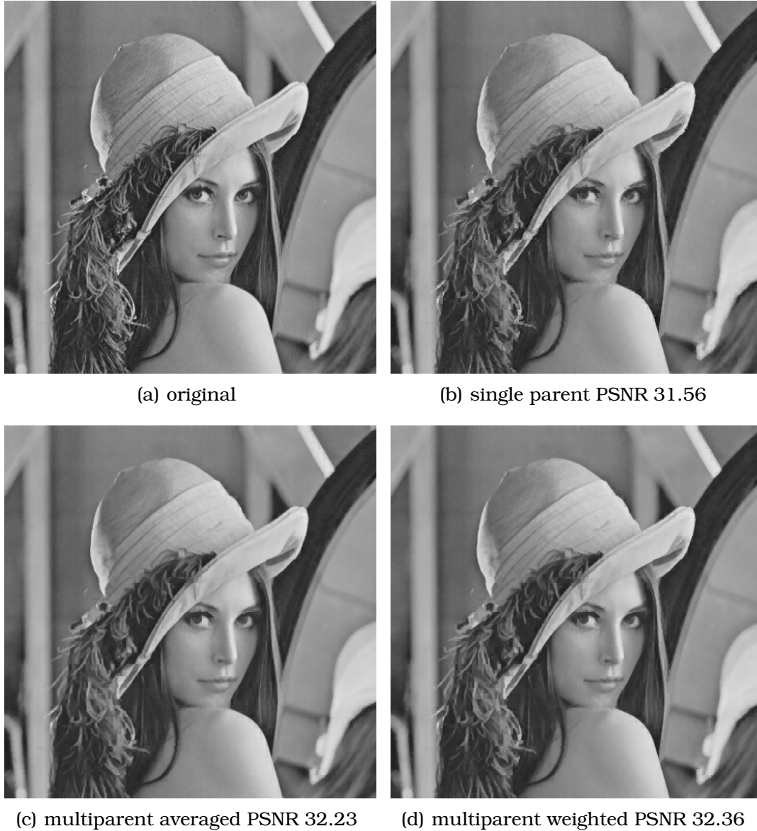
Figure 3.23: Lena partitioned into 8 \times 8 pixel range blocks. a) original b) estimated by a conventional IFS scheme c) averaged result over 10 parent blocks d) weighted average ( as 1/err^4 ) of 10 parents.
