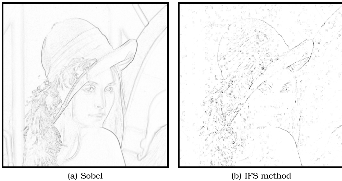
Figure 3.35: Comparison of IFSM edges with Sobel filter output.
