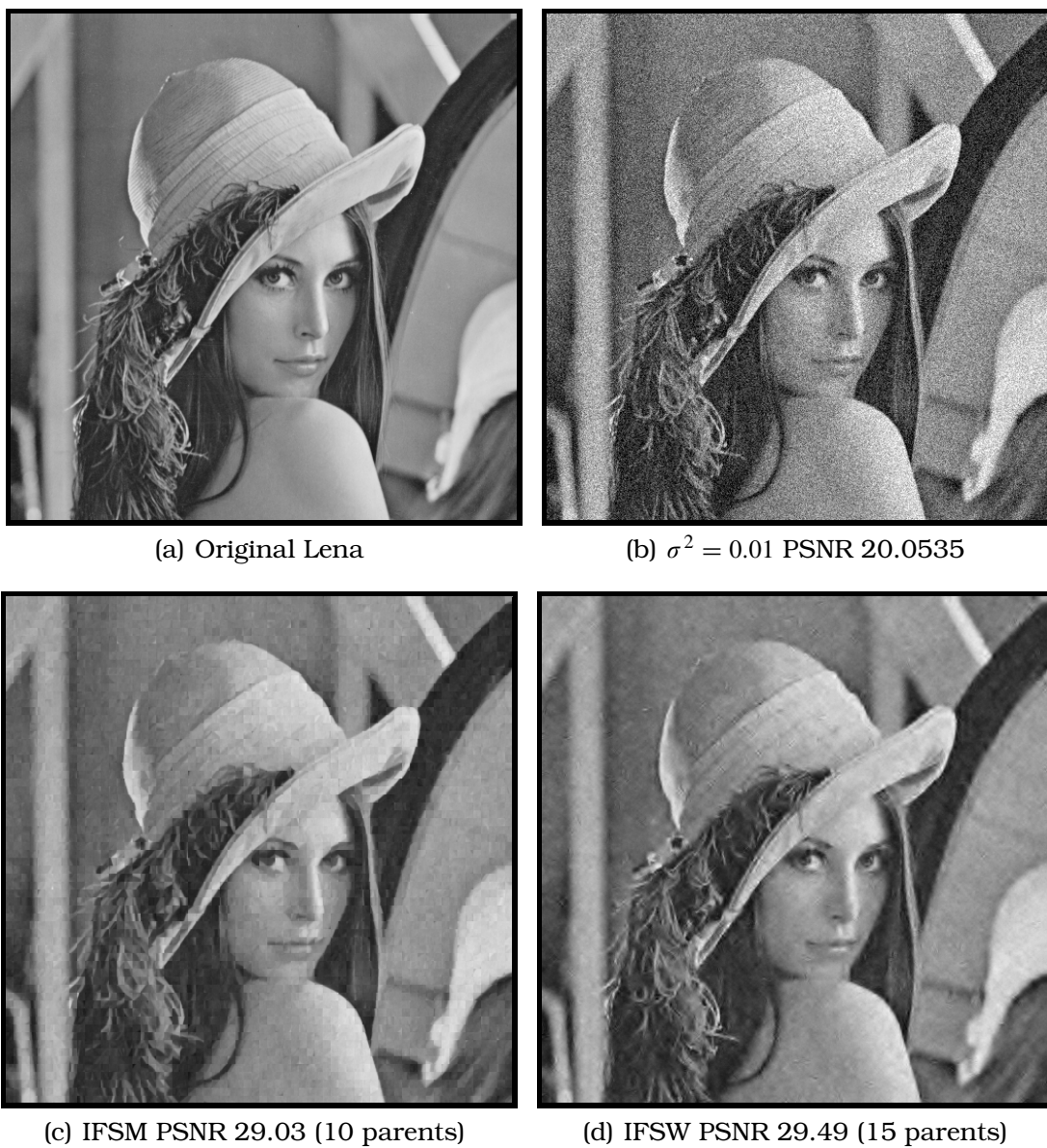
Figure 3.30: Original (a) and noisy (b) Lena images. Denoised versions using (c) spatial IFSM and (d) wavelet IFSW.
