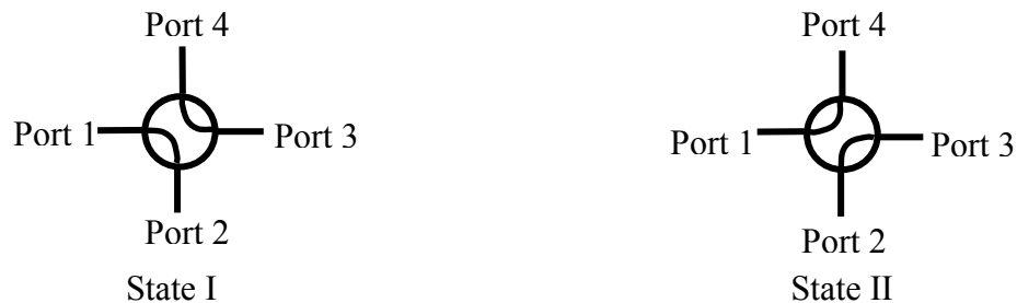
Figure 3.10: C-type switch schematic; in state I ports 1-2 & 3-4 are connected and in state II ports 1-4 & 2-3 are connected.
