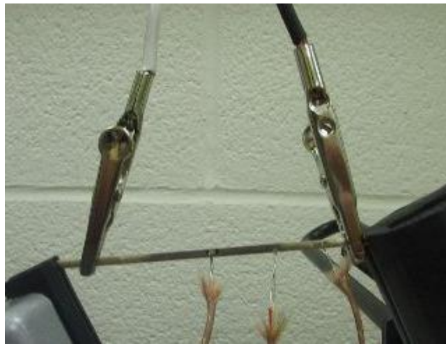
Figure 6.16: Thermocouples and electrical leads on silver-tin end-soldered Nichrome strip.
