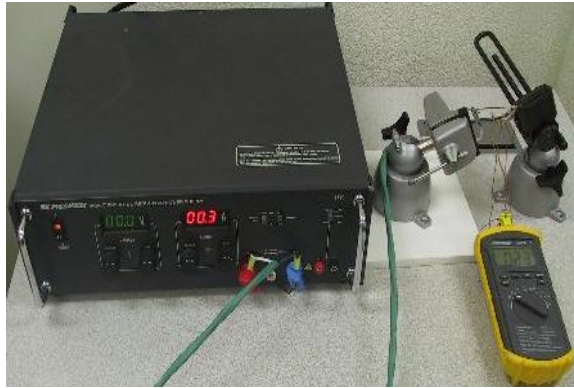
Figure 6.15: Experimental set-up for silver-tin end-soldered Nichrome strip current-to-temperature test. The 20 A direct-current power supply is on the left. The vices holding the Nichrome strip are on the right above the Omega HH501DK thermometer.
