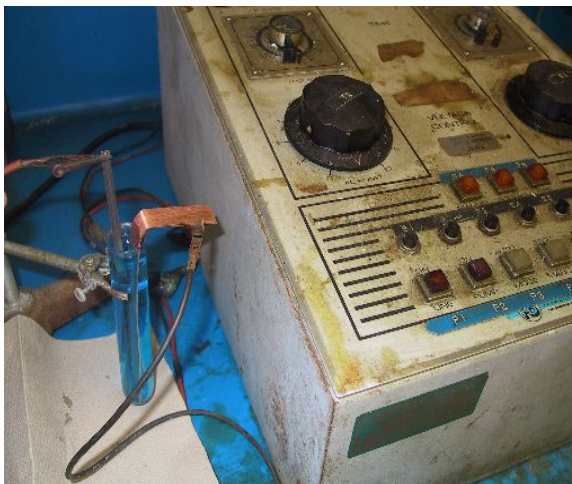
Figure 6.10: Electroplating apparatus. The power supply is on the right. The solution in the test tube is the electrolyte. Strips of Nichrome (left) and copper (right) are in the test tube.
