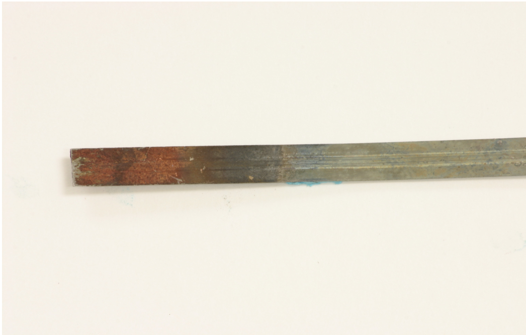
Figure 6.12: “Burned-looking” electroplated strip of Nichrome.
