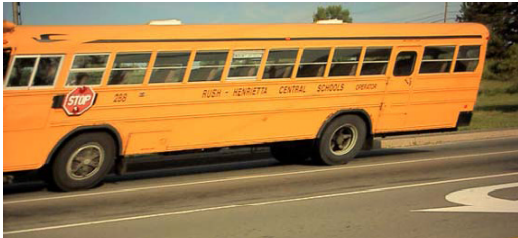
Fig 3.17 Impact of rolling-shutter on CMOS sensor causing motion blur
