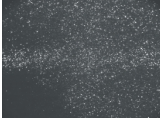
Figure 2.13: Medium image density (Turbulent opposed impinging jets - Re = 11000 , L^* = 20 ; TiO_2 particles, image 1008 \times 1018 pixels )
