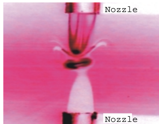
Figure 4.6: Turbulent opposed impinging jets - horizontal XY plane (LIF technique, L^* = \{5, 20\} , Re = \{100, 142000\} )
