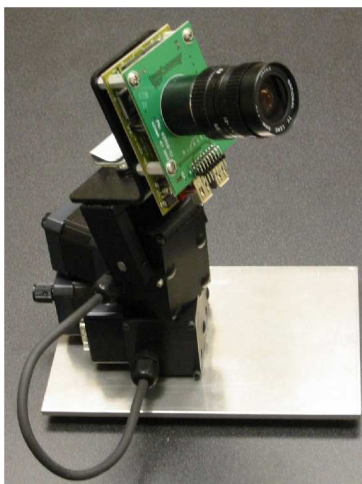
Figure 3.3: The Mike prototype consists of a commercial CMOS camera mounted on a programmable servomotor.
