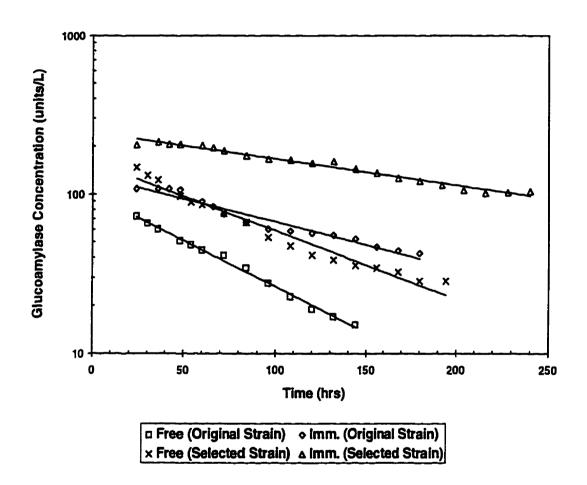
Figure 6.4. Comparison of Enzyme Concentrations between Free and Immobilized Cell Systems for Original and Selected Strains (Temperature = 30 °C, Aeration Rate = 1.0 VVM, Dilution Rate =  $0.1 \, h^{-1}$ ,  $G_0 = 20.0 \, g/L$ ).
