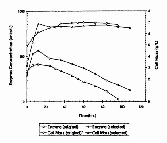
Figure 4.12. Comparison of Glucoamylase Concentration between Original and Selected Strains in Continuous Suspension Culture in Stirred-Tank Bioreactor (T = 30 °C, D = 0.1 h<sup>-1</sup>, VVM = 1.0, RPM = 500 and  $G_0 = 20.0$  g/L).
