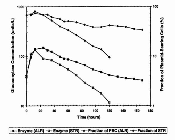
Figure 4.24. Correlation between Enzyme Production and Plasmid Loss During Continuous Culture in ALR and STR Bioreactors Using Selected Strain (D = 0.10  $h^{-1}$ , T = 30 °C, VVM = 1.0, RPM = 500 and  $G_0$  = 20.0 g/L).
