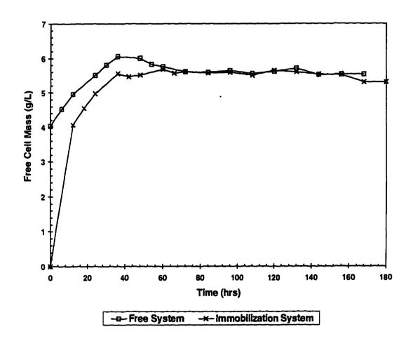
Figure 6.6. Comparison of Free Cell Mass between Free and Immobilized Cell Systems (Original Strain; Temperature = 30 °C, Aeration Rate = 1.0 VVM, Dilution Rate = 0.1  $h^{-1}$ ,  $G_0$  = 20.0 g/L).
