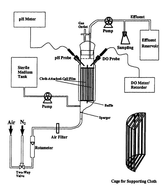
Figure 3.1. Immobilized-Cell-Film Airlift Bioreactor and Setup for Continuous Culture
