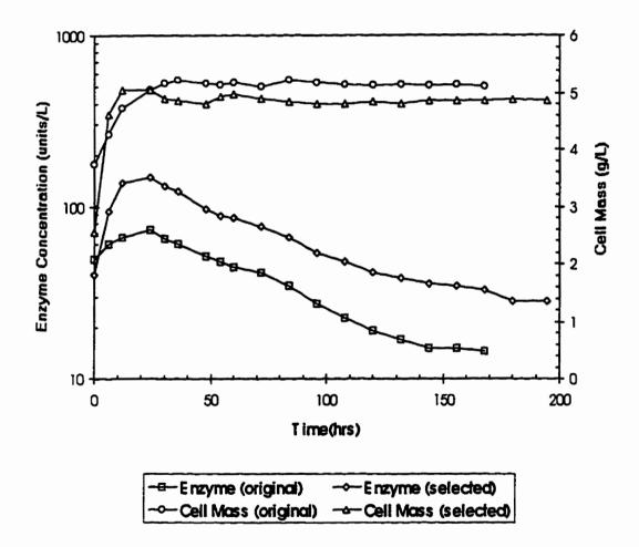
Figure 4.13. Comparison of Glucoamylase Concentrations between Original and Selected Strains in Continuous Suspension Culture in Airlift Bioreactor (T = 30  $^{\circ}$ C, D = 0.1 h<sup>-1</sup>, VVM = 1.0 and G<sub>0</sub> = 20.0 g/L).
