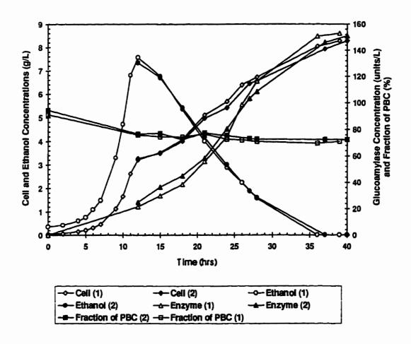
Figure 3.2. Reproducibility Check in Free Suspension Batch Fermentation (Temperature = 30 °C, Aeration Rate = 1.0 VVM).
