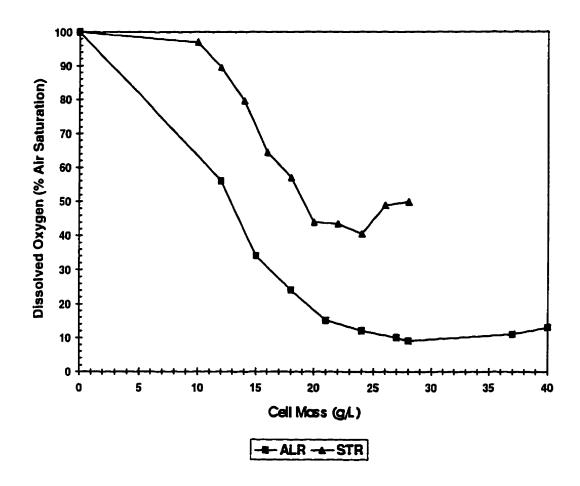
Figure 4.4. Comparison of Dissolved Oxygen Profiles between Stirred-Tank and Airlift Bioreactors.
