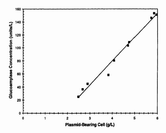
Figure 5.1. Linear Regression of Glucoamylase Concentration to Plasmid-Bearing Cell Concentration in Batch Culture in Airlift Bioreactor.
