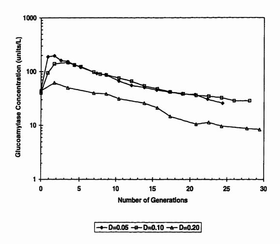
Figure 4.19. Effects of Dilution Rate and Generation Number on Glucoamylase Expression during Continuous Culture in Airlift Bioreactor (T = 30 °C, VVM = 1.0 and  $G_0 = 20.0$  g/L).
