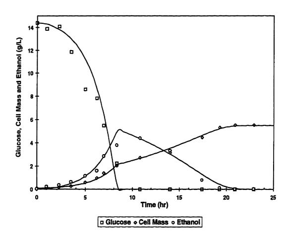
Figure 5.4. Comparison between Model Simulation (solid line) and Experimental Data (markers) for Batch Fermentation with Recombinant Yeast Strain SEY2102/pRB58 Producing Invertase (data from Parker and Seo (1992).
