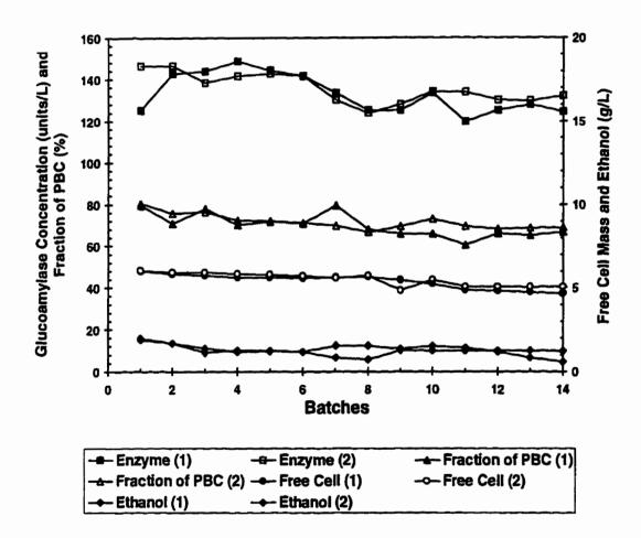
Figure 3.5. Reproducibility Check in Repeated Batch Fermentation with Immobilized Cell System (Temperature = 30 °C, Aeration Rate = 1.0 VVM).
