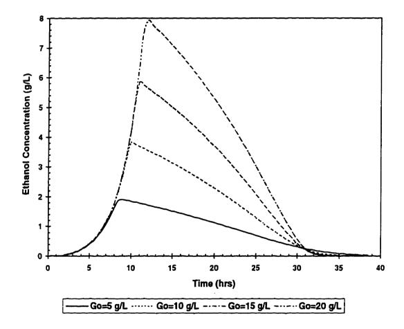
Figure C.3. Effect of Initial Glucose Concentration on Ethanol Concentration in Batch Culture.
