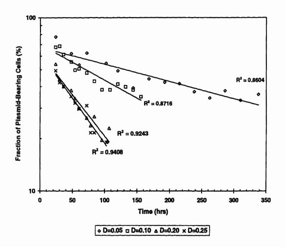
Figure 4.14. Effects of Dilution Rate and Time on Plasmid Stability during Continuous Culture in Airlift Bioreactor Using Nonselective Medium (T = 30 °C, VVM = 1.0 and  $G_0 = 20.0$  g/L).
