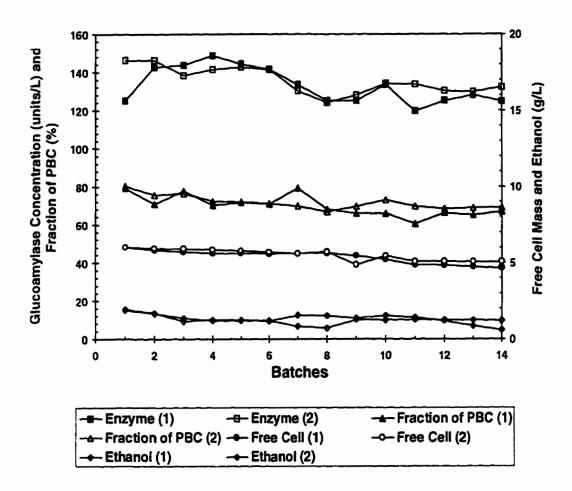
Figure 6.12. Results for Two Repeated Batch Fermentation Experiments in Immobilized-Cell-Film Airlift Bioreactor. (Selected Strain; Temperature = 30 °C, Aeration Rate = 1.0 VVM, Each Batch Lasted 24 hours).
