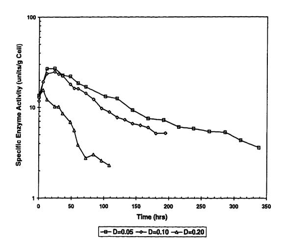
Figure 4.21. Effects of Dilution Rate on Specific Enzyme Activity during Continuous Culture in Airlift Bioreactor (T = 30  $^{\circ}$ C, VVM = 1.0 and G<sub>0</sub> = 20.0 g/L).
