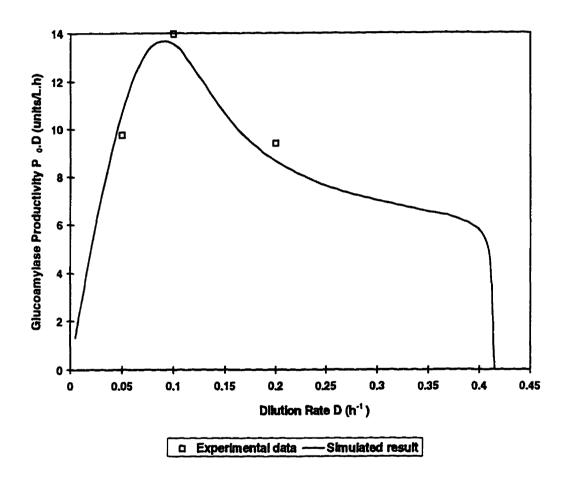
Figure 5.6. Effect of Dilution Rate on Glucoamylase Productivity during Continuous Fermentation in Airlift Bioreactor with Recombinant Yeast Strain C468/pGAC9 Producing Glucoamylase.
