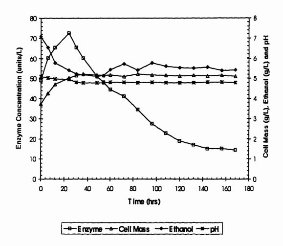
Figure 4.9. Continuous Suspension Culture in Airlift Bioreactor Using Original Strain at  $T=30\,^{\circ}C$ ,  $D=0.1\,h^{-1}$ , VVM = 1.0 and  $G_0=20.0\,g/L$ .
