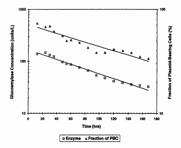
Figure 4.26. Correlation between Fraction of Plasmid-Bearing Cells and Enzyme Concentration during Continuous Culture in ALR Bioreactor Using Nonselective Medium (D =  $0.10 \; h^{-1}$ , VVM = 1.0, T =  $30 \; ^{\circ}$ C and  $G_0 = 20 \; g$  /L).
