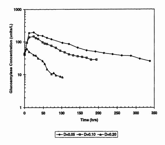
Figure 4.18. Effects of Dilution Rate and Time on Glucoamylase Expression during Continuous Culture in Airlift Bioreactor (T = 30  $^{\circ}$ C, VVM = 1.0 and G<sub>0</sub> = 20.0 g/L).
