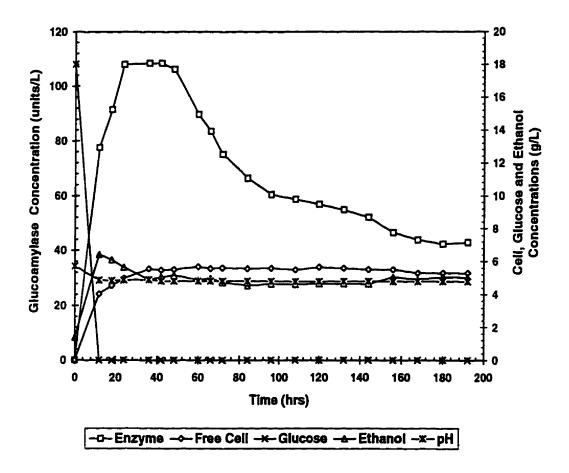
Figure 6.2. Continuous Recombinant Yeast Fermentation in Immobilized-Cell-Film Bioreactor Using Original Strain. Temperature = 30 °C, Aeration rate = 1.0 VVM, Dilution rate =  $0.1 \, h^{-1}$ ,  $G_0 = 20.0 \, g/L$ .
