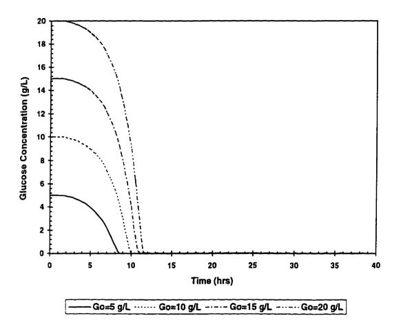
Figure C.1. Effect of Initial Glucose Concentration on Residual Glucose in Batch Culture.
