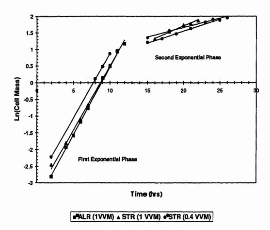
Figure 4.5. Determination of Specific Growth Rates by Semilogarithmic Plot of Cell Concentration versus Time in Two Different Exponential Growth Phases.
