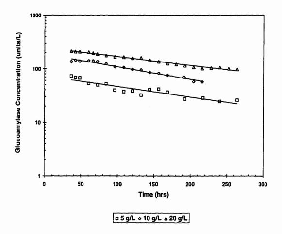
Figure 6.10. Effect of Glucose Feed Concentration ( $G_0$ ) on Enzyme Production in Immobilized Cell System at Dilution Rate = 0.1 h<sup>-1</sup>. (Selected Strain; Temperature = 30 °C, Aeration Rate = 1.0 VVM)
