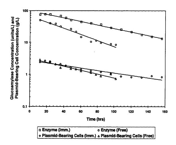
Figure 6.8. Comparison of Plasmid Loss and Glucoamylase Production between Free and Immobilized Cell Systems at Dilution rate =  $0.2 \, h^{-1}$ . (Selected Strain; Temperature =  $30 \, ^{\circ}$ C, Aeration Rate =  $1.0 \, \text{VVM}$ ,  $G_0 = 20.0 \, \text{g/L}$ ).
