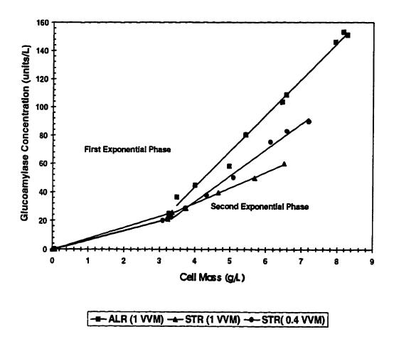
Figure 4.6. Determination of Recombinant Protein Yield by Linear Regression of Glucoamylase Concentration with regard to Cell Concentration in Two Different Exponential Growth Phases.
