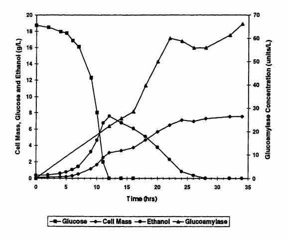
Figure 4.2. Typical Time Course of Batch Culture in Stirred-Tank Bioreactor.
