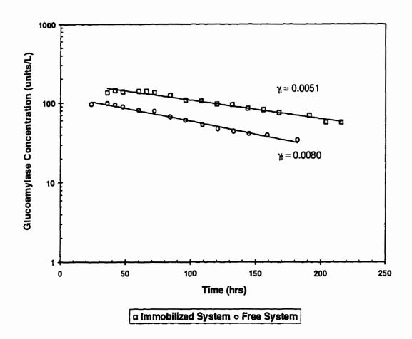
Figure 6.9. Comparison of Glucoamylase Concentration between Free and Immobilized Cell System at Glucose Feed Concentration ( $G_0$ ) = 10 g/L and Dilution Rate = 0.1 h<sup>-1</sup>. (Selected Strain; Temperature = 30 °C, Aeration Rate = 1.0 VVM).
