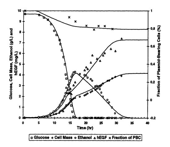
Figure 5.3. Comparison between Model Simulation (solid line) and Experimental Data (markers) for Batch Fermentation with Recombinant Yeast Strain AB103.1/pYαEGF-25 Producing Human Epidermal Growth Factor (data from Coppella and Dhurjati (1990)).
