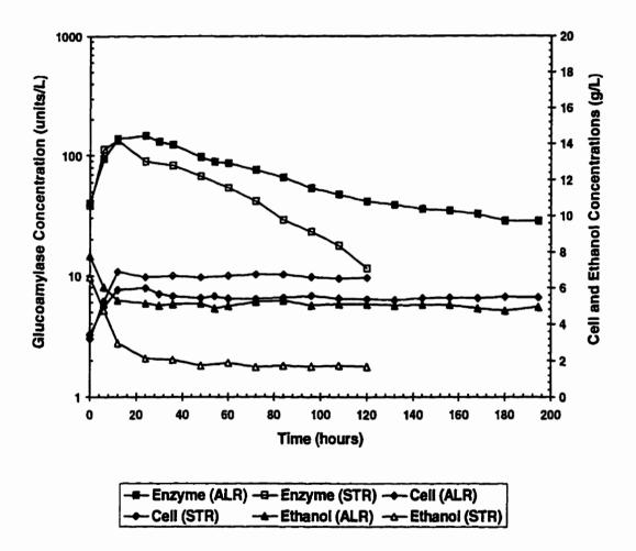
Figure 4.23. Comparisons of Enzyme, Cell and Ethanol Concentrations between ALR and STR Bioreactors in Continuous Culture Using Selected Strain (D = 0.10  $h^{-1}$ , T = 30 °C , VVM = 1.0, RPM = 500 and  $G_0$  = 20.0 g/L).
