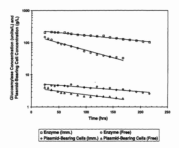
Figure 6.7. Comparison of Plasmid Loss and Glucoamylase Production between Free and Immobilized Cell Systems at Dilution rate =  $0.1 \, h^{-1}$ . (Selected Strain; Temperature =  $30 \, ^{\circ}$ C, Aeration Rate =  $1.0 \, \text{VVM}$ ,  $G_0 = 20.0 \, \text{g/L}$ ).
