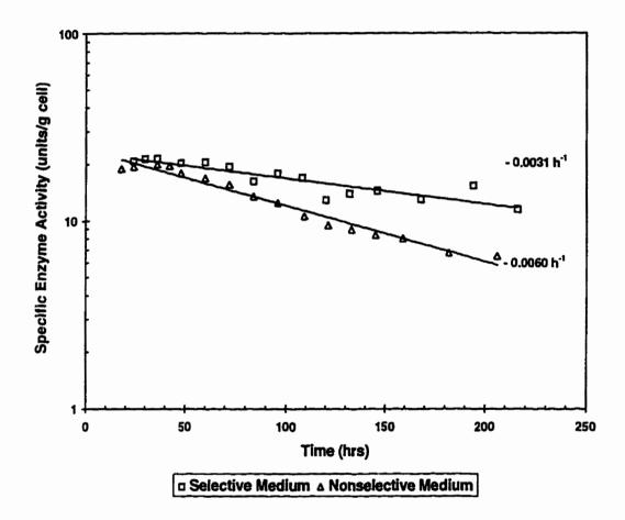
Figure 4.27. Comparison of Specific Enzyme Activity between Selective and Nonselective Media during Continuous Culture in ALR (D = 0.10  $h^{-1}$ , VVM = 1.0, T = 30 °C,  $G_0 = 10$  /L).
