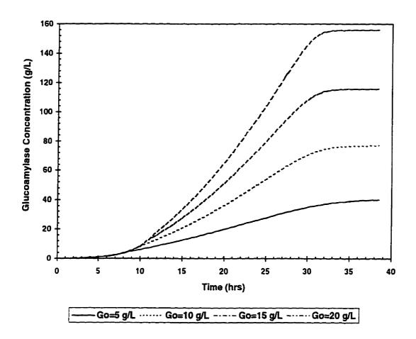
Figure C.4. Effect of Initial Glucose Concentration on Glucoamylase Concentration in Batch Culture.
