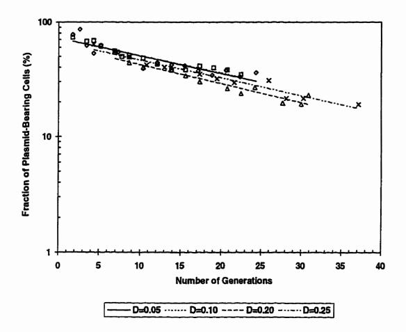
Figure 4.15. Effects of Dilution Rate and Generation Number on Plasmid Stability during Continuous Culture in Airlift Bioreactor Using Nonselective Medium (T = 30°C, VVM = 1.0 and  $G_0 = 20.0$  g/L).
