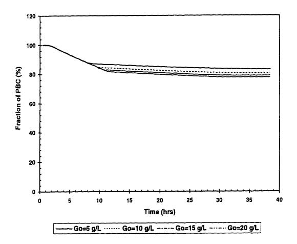
Figure C.5. Effect of Initial Glucose Concentration on Fraction of Plasmid-Bearing in Batch Culture.
