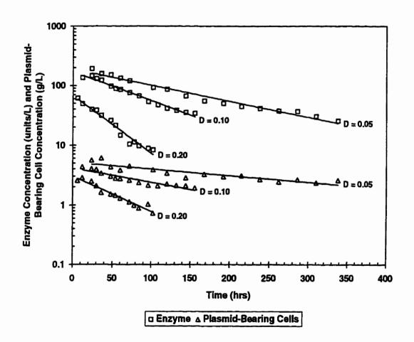
Figure 5.8. Relationship between Plasmid-Bearing Cell Concentration and Glucoamylase Concentration in Continuous Suspension Culture of Recombinant Yeast Strain C468/pGAC9.
