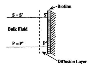
Figure 6.1. Schematic Diagram of Idealized Biofilm.
