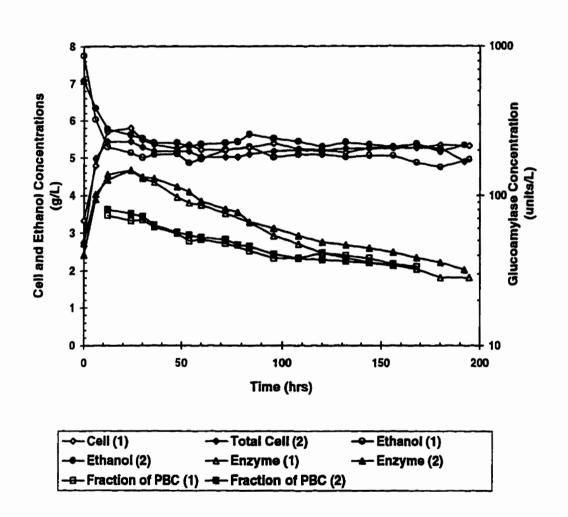
Figure 3.3. Reproducibility Check in Free Suspension Continuous Fermentation (Temperature = 30 °C, Aeration Rate = 1.0 VVM, Dilution Rate = 0.1 h<sup>-1</sup>).
