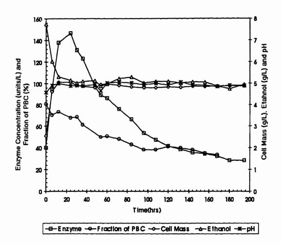
Figure 4.11. Continuous Suspension Culture in Airlift Bioreactor Using Selected Strain at T = 30 °C,  $D = 0.1 \, h^{-1}$ , VVM = 1.0 and  $G_0 = 20.0 \, g/L$ .
