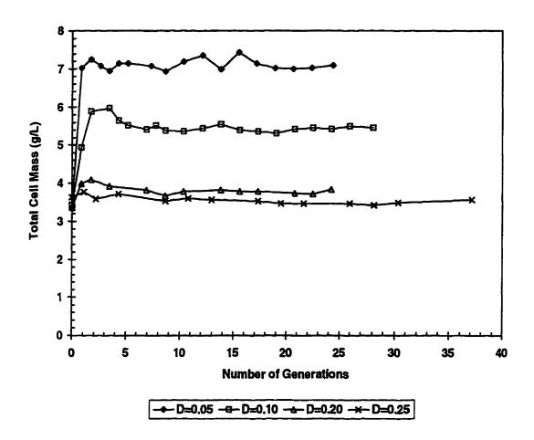
Figure 4.17. Total Cell Mass at Different Dilution Rates during Continuous Culture Process (T = 30  $^{\circ}$ C, VVM = 1.0 and G<sub>0</sub> = 20.0 g/L).
