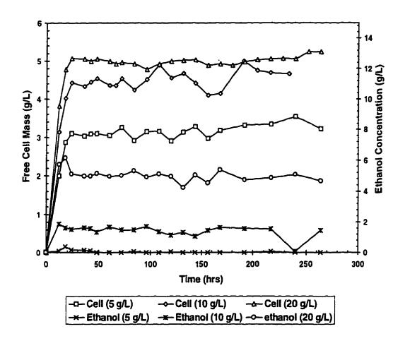
Figure 6.11. Effect of Glucose Feed Concentration ( $G_0$ ) on Free Cell Mass and Ethanol Concentration in Immobilized Cell System at Dilution Rate = 0.1 h<sup>-1</sup>. (Selected Strain; Temperature = 30 °C, Aeration Rate = 1.0 VVM)
