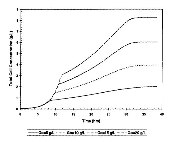
Figure C.2. Effect of Initial Glucose Concentration on Total Cell Concentration in Batch Culture.
