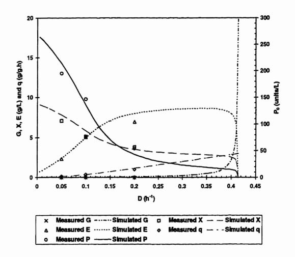
Figure 5.5. Effect of Dilution Rate on G, X, E, q and  $P_0$  during Continuous Fermentation in Airlift Bioreactor with Recombinant Yeast Strain C468/pGAC9 Producing Glucoamylase.
