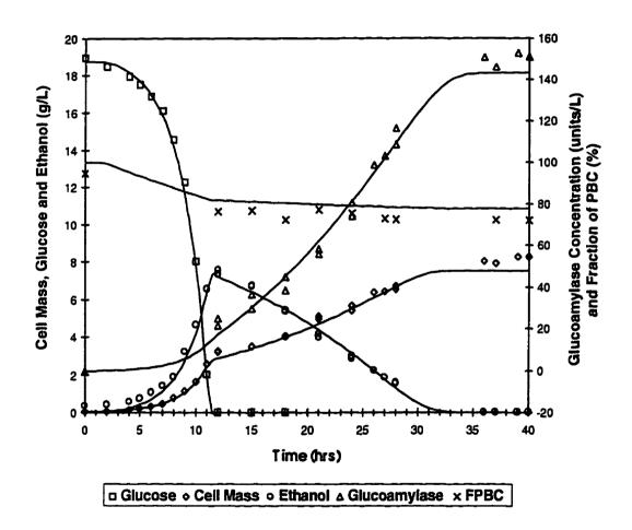
Figure 5.2. Comparison between Model Simulation (solid line) and Experimental Data (markers) for Batch Fermentation with Recombinant Yeast Strain C468/pGAC9 Producing Glucoamylase (data from current studies).
