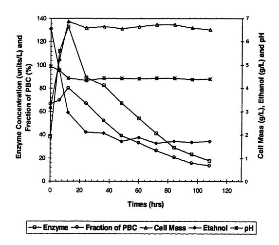
Figure 4.10. Continuous Suspension Culture in Stirred-Tank Bioreactor Using Selected Strain at T=30 °C, D=0.1 h<sup>-1</sup>, VVM = 1.0, RPM = 500 and  $G_0=20.0$  g/L.
