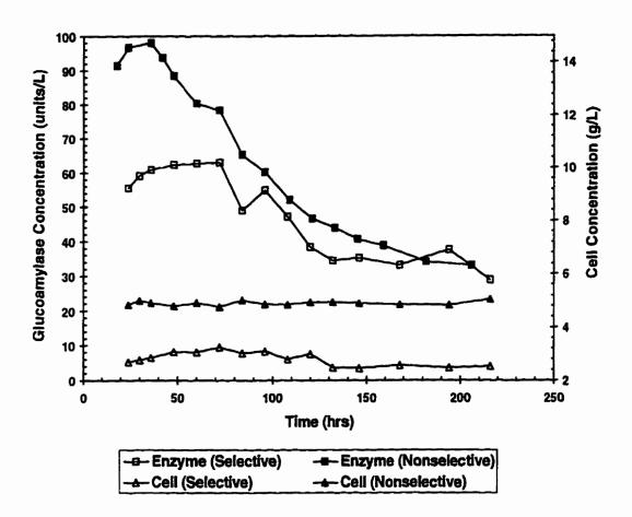
Figure 4.28. Comparison of Cell Mass and Enzyme Concentration between Selective and Nonselective Media during Continuous Culture in ALR (D = 0.10  $h^{-1}$ , VVM = 1.0, T = 30 °C and  $G_0$  = 10 /L).
