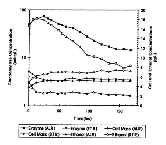
Figure 4.22. Comparisons of Enzyme, Cell and Ethanol Concentrations between ALR and STR Bioreactors in Continuous Culture Using Original Strain (D = 0.10  $h^{\text{-1}},\,T=30\,^{\circ}\text{C}$ , VVM = 1.0, RPM = 500 and  $G_0=20.0$  g/L).
