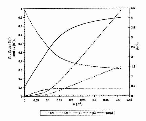
Figure 5.7. Effect of Dilution Rate on  $C_I$ ,  $C_2$ ,  $\mu_1$ ,  $\mu_2$  and  $\mu_1/\mu_2$  during Continuous Fermentation in Airlift Bioreactor with Recombinant Yeast Strain C468/pGAC9.
