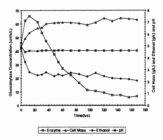
Figure 4.8. Continuous Suspension Culture in Stirred-Tank Bioreactor Using Original Strain at  $T=30\,^{\circ}C$ ,  $D=0.1\,h^{-1}$ , VVM=1.0, RPM=500 and  $G_0=20.0$  g/L.
