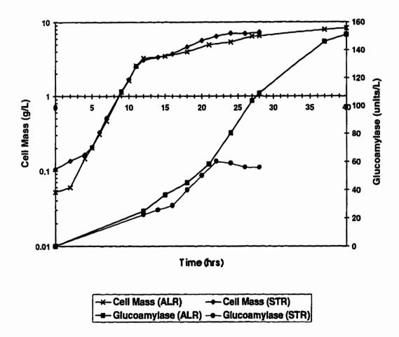
Figure 4.3. Comparison of Cell and Glucoamylase Concentrations between Stirred-Tank and Airlift Bioreactors.
