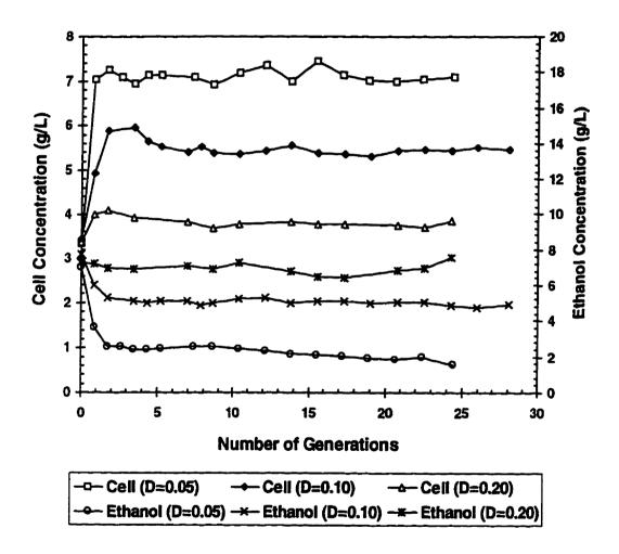
Figure 4.20. Effects of Dilution Rate on Cell and Ethanol Concentrations during Continuous Culture in Airlift Bioreactor (T = 30 °C, VVM = 1.0 and  $G_0 = 20.0$  g/L).
