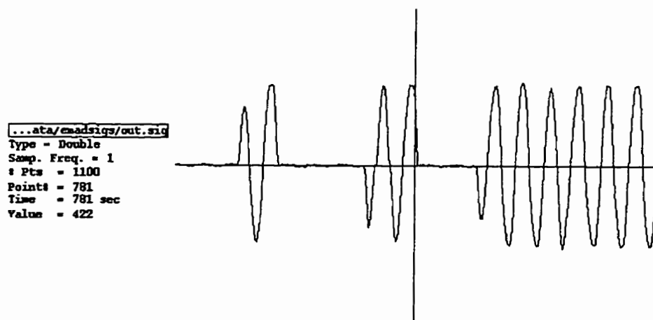
Figure 5.16: Distortion in the output signal of the bandpass Sigma-Delta modulator shown in Figure 5.7.a due to G_{loope} = 1.0 and G_{loopo} = 0.95 .
