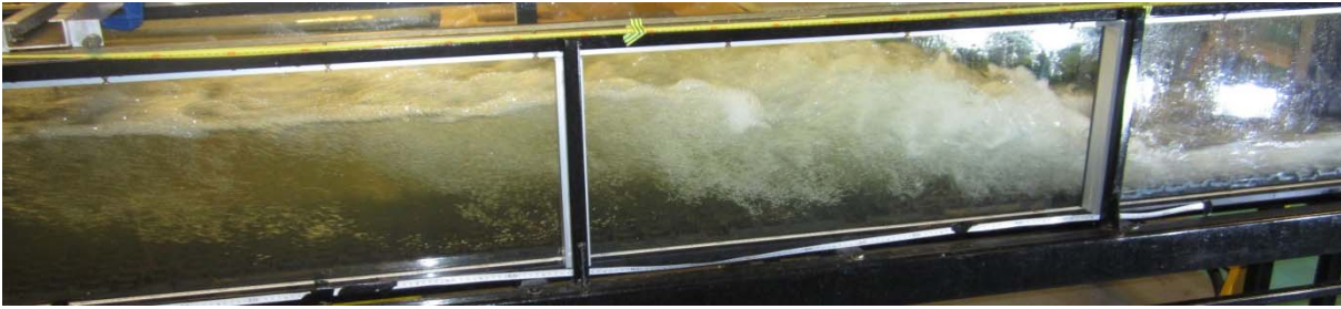
Fig. 4. Hydraulic jumps on bed roughness configuration 2
