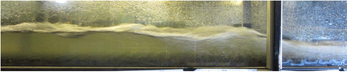
Fig. 4. Hydraulic jumps on bed roughness configuration 2
