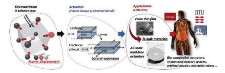
Despite this great potential, so far only CGO thin films with a specific textured microstructure have been found to be electromechanically active. With this in mind, the scientific aim of the GIANT-E project is to unveil the inner mechanism governing the electrostriction effect in these materials, and extend such property to the bulk form. The technological aim is to stabilize the electrostriction effect in thick samples, for a new paradigm of lead-free electromechanical active materials.
