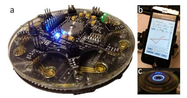
The first application of the PLoD is a potentiostat for electrochemical based biosensing [1], we have successfully measure Ferri Ferrocyanides Current-Potentio curve while spinning from 0 to 3000 rpm. There are various lab-on-disc applications[2] can be carry out by the PLoD platforem for the future stand-along diagnostics and healthcare systems.
