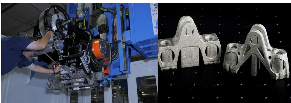
Left: Loading metal foil to an additive manufacturing welding machine (source: Fabrisonic)
