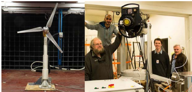
Figure 1: (Left) The model wind turbine and the Lidic lidar telescope on a traversing system in the background. (Right) One of the short-range WindScanners surrounded by some of the authors.
