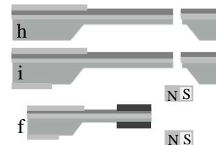
Figure 3. Beam released and bottom electrode deposition (h-i). Ferromagnetic foils and magnets are incorporated (f).
