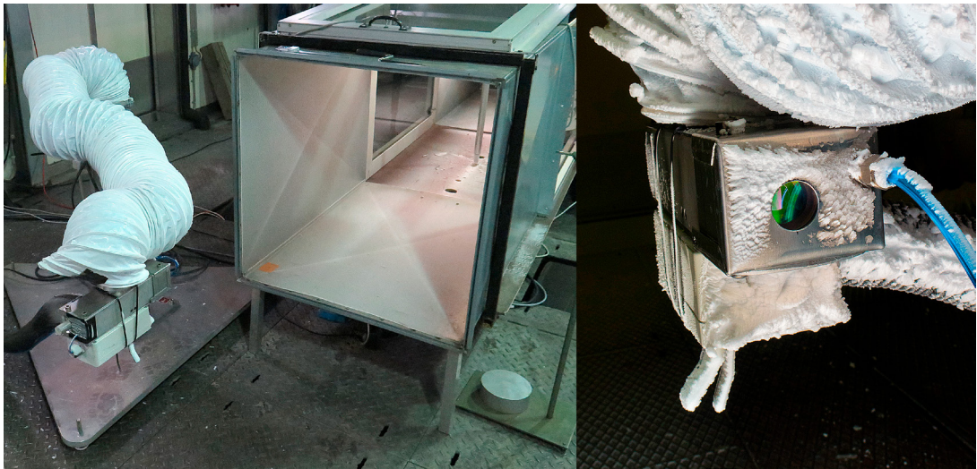
Fig. 2. (Left) The Lidar telescope (Lidic) on a robotic arm in the icing wind tunnel. (Right) Lidic with an ice prevention system that keeps the optical window free from ice and water.
