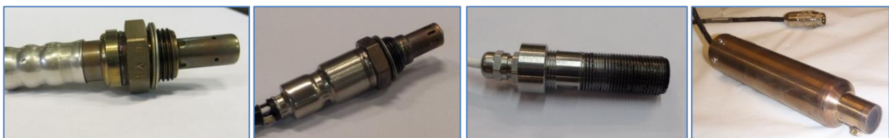
Figure 1: Evaluated sensors: NGK lambda probes OZA685-WW1 & ZFAS-U2, SenSiC CO/O 2 probe, Lamtec KS1D (from left to right)
