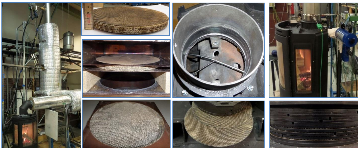
Figure 30: Catalyst test rig (left); mesh catalyst (new, in test rig, aged), new stove socket and stove integrated catalyst test set-up (right) including placement of mesh pieces (right, below)
