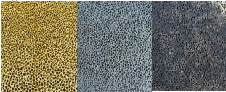
Figure 33: Foam ceramic filters applied: unused element (left), 200 batches (middle), 550 batches (right)
