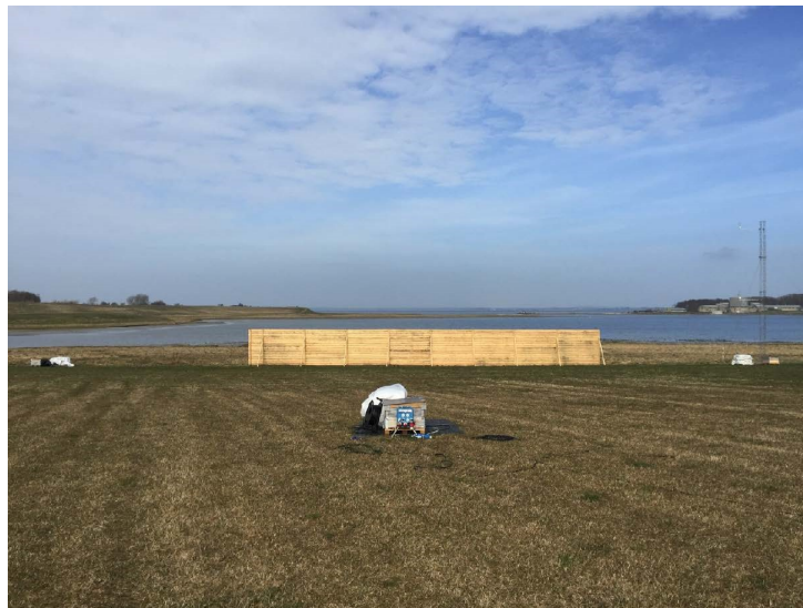
Figure 6. The fence experimental set-up at DTU Risø campus test station, installed with three short-range WindScanner lidar instruments and a met mast.
