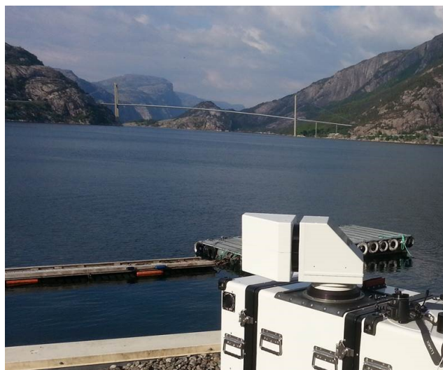
Figure 5. A long-range WindScanner operated by Christian Mikkelsen Research (CMR) during the 2014 Lysefjord bridge measurement campaign.
