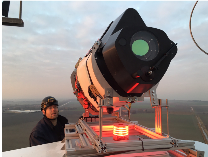
Figure 13. A DTU SpinnerLidar installed on the Nacelle of a Nordex 80 test turbine at the ECN test site in Holland during IRPWind ScanFlow 2016-2017 [22].
