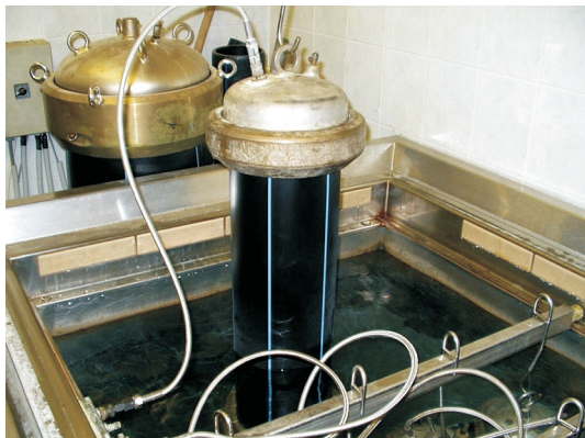
Figure 3 Mounting of pipe specimen into hot water tank [6] Slika 3. Uranjanje ispitnog tijela u toplu vodu [6]
