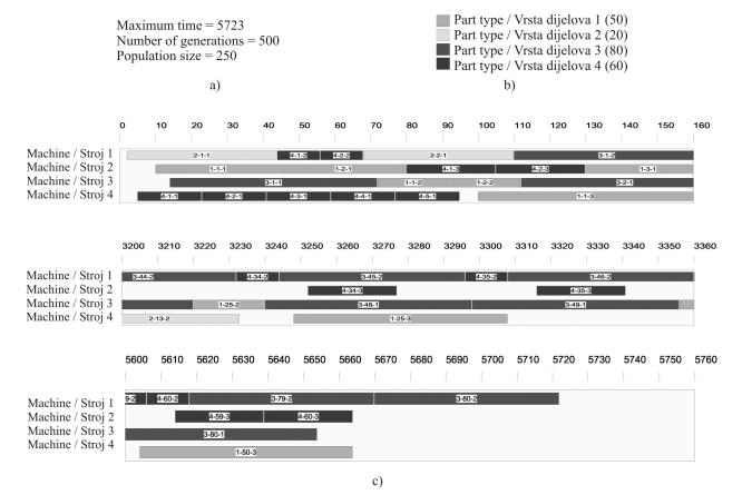
**Figure 7.** Partial presentation of task results for the minimum manufacturing cycle criterion – case 1 with GJOB program: a) result; b) legend; c) gantogram
