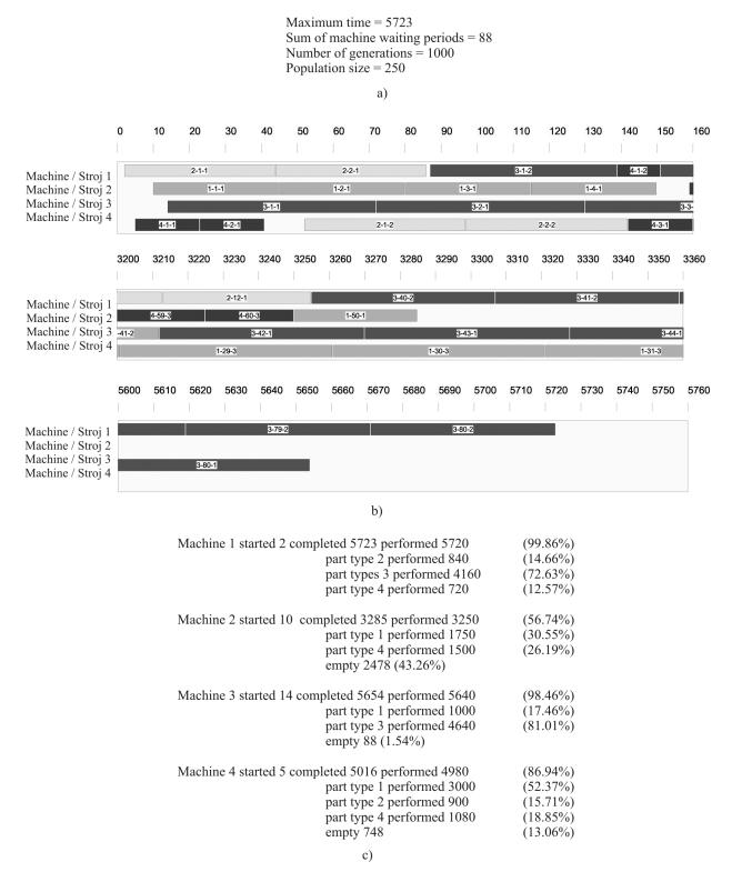
**Figure 8.** Partial presentation of task results for criteria combination – case 2 with GJOB program: a) result; b) machine gantogram; c) machine statistics
