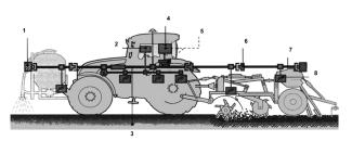
**Figure 9.** Communication between tractor and implement using ISO Bus: 1. Bus terminator, 2. Tractor internal monitor, 3. Tractor internal Bus, 4. Bus terminal, 5. Data transfer to management computer, 6. Bus connector, 7. Tractor implement Bus, 8. Electronic control unit (ECU)
