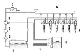
Figure 1. Common rail fuel system:
