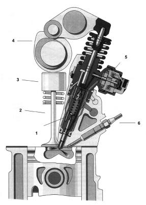
Figure 2. Nozzle-pump system 1. Nozzle, 2. Valve, 3. Cam follower, 4. Cam shaft, 5. Solenoid, 6. Glow plug
