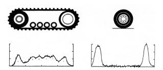
Figure 11. Contact pressure at tractor with rubber belt and wheels
