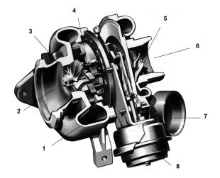
**Figure 3.** Variable geometry turbocharger (VGT): 1. Exhaustinlet, 2. Exhaust-outlet, 3. Turbine wheel, 4. Moveble vanes, 5. Charger wheel, 6. Air intlet 7. Air-outlet, 8. Membrane actuator
