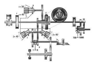
**Figure 4.** Continuously variable transmission (CVT): 1. Torsional vibration damper, 2. Planetary gear set, 3. Ring gear, 4. Sun gear, 5. Planet carrier, 6. Hydraulic pump, 7. Hydraulic motor, 8. Collecting shaft, 9. Travel range selector
