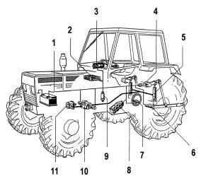
**Figure 5.** Digital Electronic-hydraulic Hitch Control System: 1. Power supply, 2. Electronic Control Unit, 3. Control panel, 4. Position sensor, 5. Hydraulic lift cylinder, 6. Draft sensor, 7. Inductive speed sensor, 8. Radar sensor, 9. Pressure sensor, 10. Hitch contlol valve, 11. Hydraulic pump
