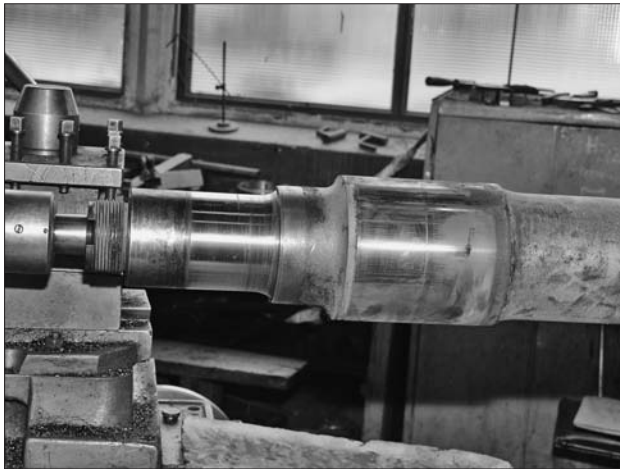
Figure 1. Damaged trunnion of a wagon axle
