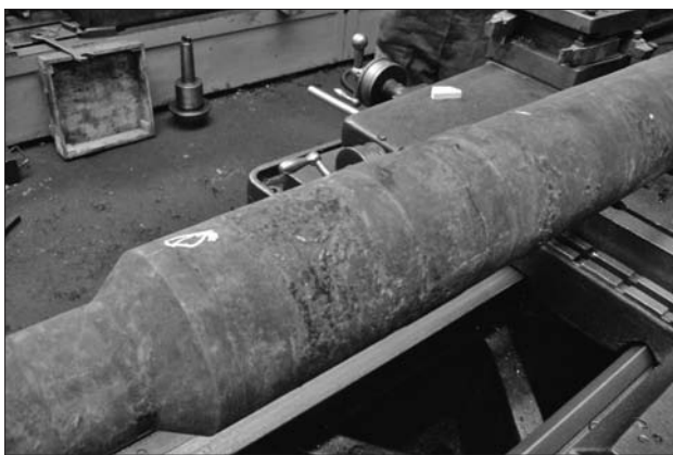
Figure 2. Damaged shaft of the screw press
