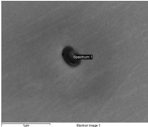
Figure 3. A Ti(C,N) inclusion in the sample of non-oriented electrical steel sheet containing 0,008 mas.% Ti
