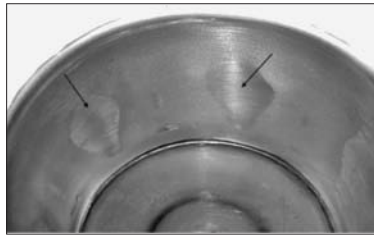
Figure 6. A defective draw piece
