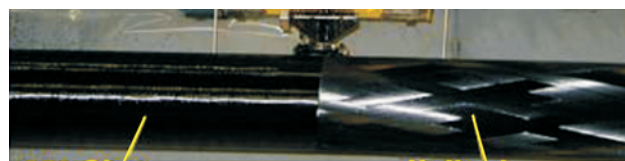
Slika 3 Obodno i vijčano namotavanje [6] Figure 3 Filament and helical winding [6]
