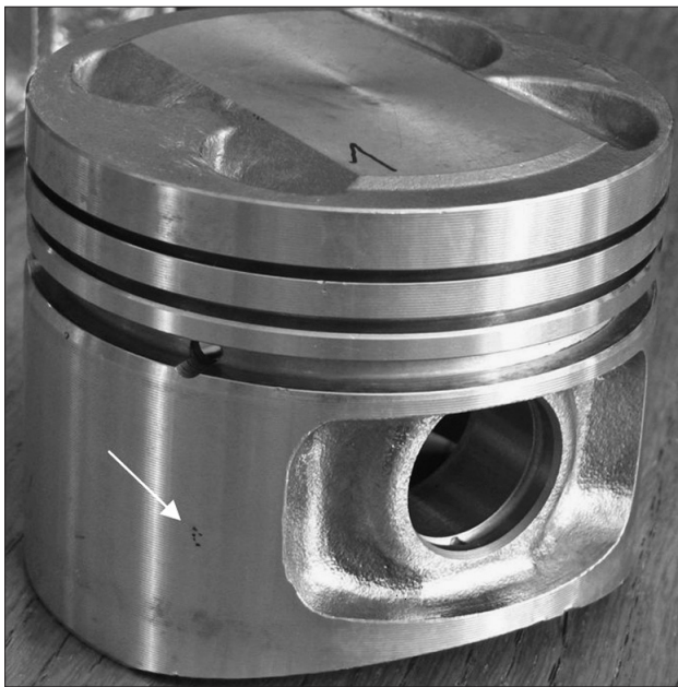
Figure 1. Machined piston with found porosity – see arrow
