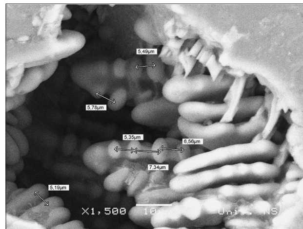
Figure 7. Secondary electron image of the type B porosity
