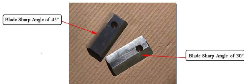
Figure 2: The Developed Blades with Angles of 30° and 45°
