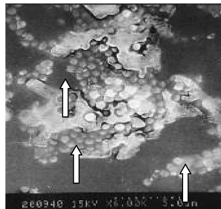
Fig. 1 – SEM images taken of BFs produced by Bacillus sp. F6 ( \times 6000 ). Arrowheads indicate the biologically produced flocculants.
