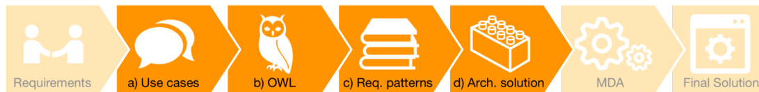
Figure 1.3: The SCenario bAsed Rapid software Prototyping (SCARP) approach, as part of a model driven development process.
