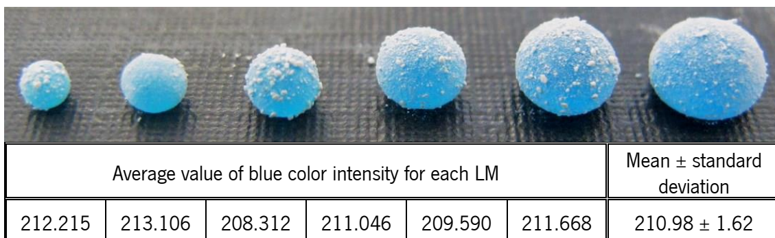
Figure 7.S1: Liquid marbles (LM) with distinct sizes produced from liquid droplets with the following volumes: 5, 7.5, 10, 20, 30 and 40 \mu\text{L} . The average value of blue color intensity was determined by ImageJ for each LM, the whole area of each LM was used for the determination. The mean value of all six values was calculated as well as the respective standard deviation.
