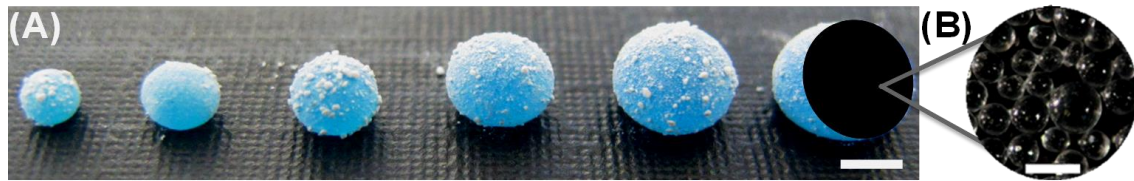
Figure 7.3: (A) Liquid marbles with distinct sizes produced from liquid droplets with the following volumes: 5, 7.5, 10, 20, 30 and 40 \mu\text{L} . Scale bar is 1 mm. (B) Optical microscopy image of PLLA microparticles that were dispersed in the core of the liquid marbles to provide anchorage sites for cell adhesion. Scale bar is 100 \mu\text{m} .
