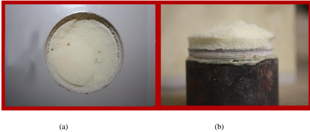
Fig. 4.11. Pull-off test failure: (a) failure in the PU foam core of sandwich panel; (b) aluminum disk.
