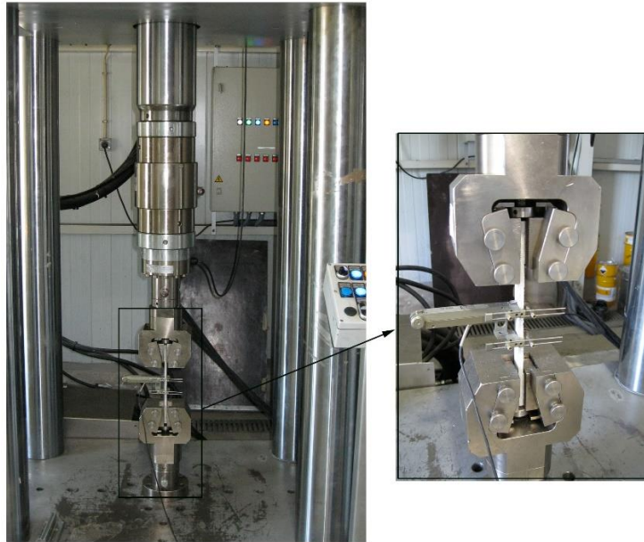
Fig. 4.2. GFRP tension test.
