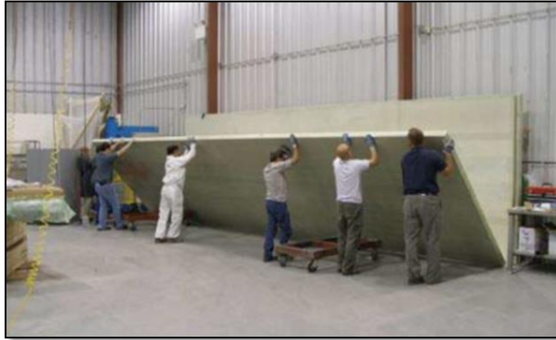
Fig. 2.10. Typical full-scale sandwich composite cladding Wall [38].
