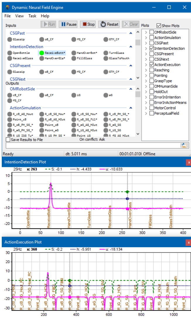
Fig. 3. Engine with Intention Detection and Action Execution neural fields plots. S , h , and u are the neural field input, resting level, and activation, respectively.
