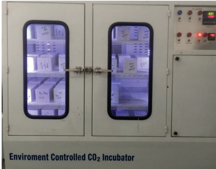
Fig. 3(a) Accelerated environment controlled carbonation chamber
