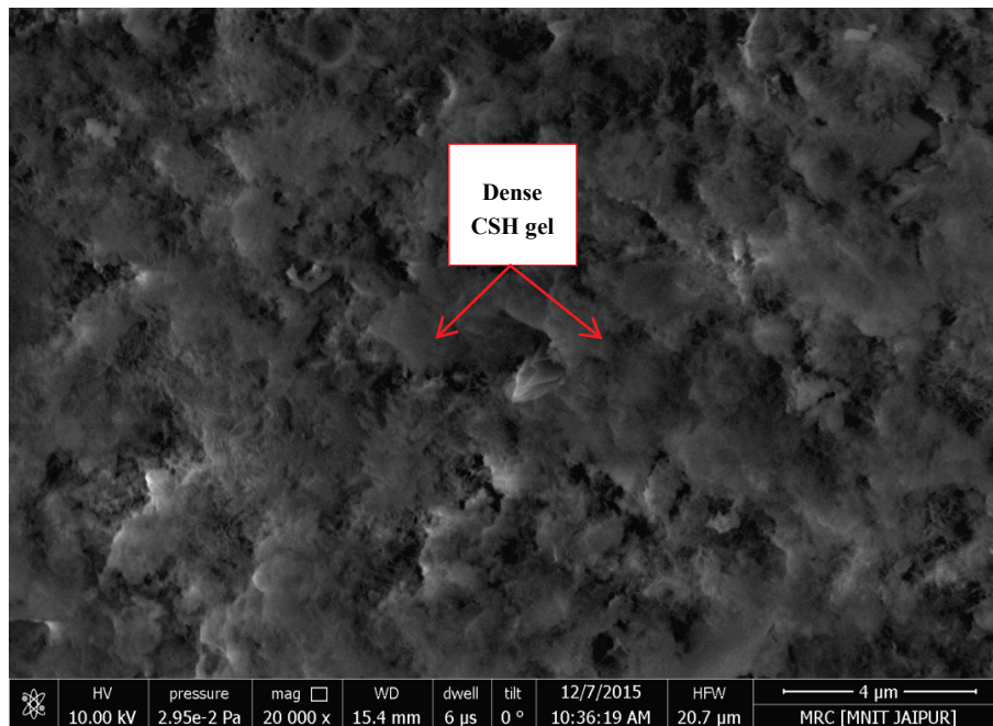
Fig. 9 SEM photograph showing dense formation of CSH gel after 90 days of curing
